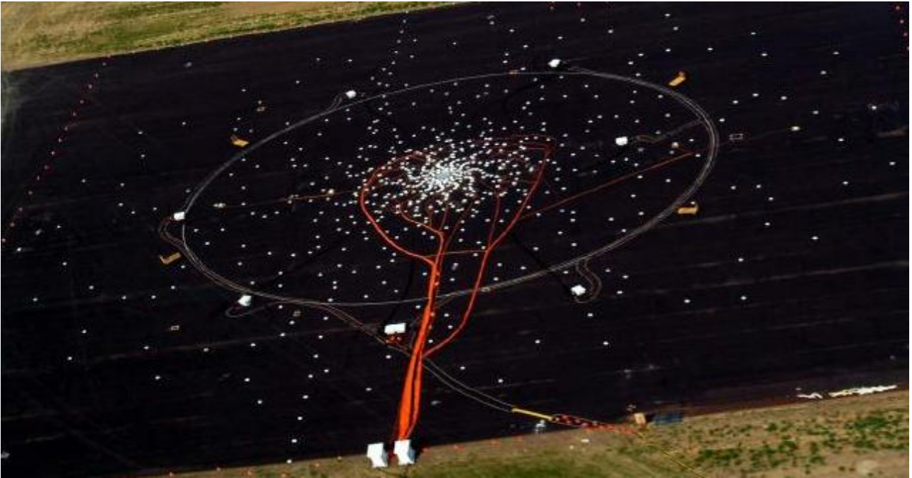
Figure 3. Boeing 2D Array of Microphones Placed on a Runway
